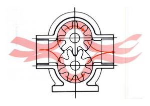
Liquid flows into the pump through the inlet (suction) branch (screwed or flanged connection); is carried round by the rotating rotors and pumped out of the outlet (delivery) port (screwed or flanged connection) . Contact between the gear teeth separates and seals the suction side from the delivery side of the pump. This creates the vacuum which allows atmospheric pressure or a positive suction head to get the liquid into the pump.
