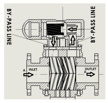
In the diagram normal flow is shown with arrow (A), the fluid flows through the pump suction and out of the delivery branch at the required pressure.
