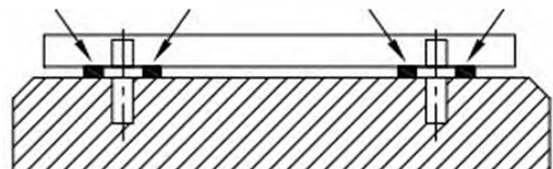
Fig.2 Foundation, baseplate and fitting the shims
