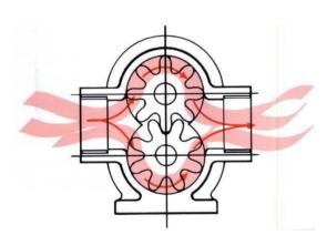
Liquid flows into the pump through the inlet (suction) branch (screwed or flanged connection); is carried round by the rotating rotors and pumped out of the outlet (delivery) port (screwed or flanged connection)
